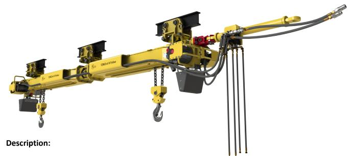
Hydraulic transport equipment TZHK2x5, hereinafter referred to as the transport equipment, is a equipment used to transport and handle loads on a single-track suspension track located in the mine section and on the surface in a horizontal plane and in inclinations up to ±30°.
